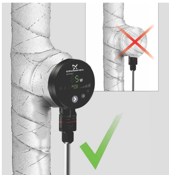
Fig. 6 Insulation of pump housing
