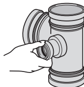
Fig.24c Positioning adaptor
