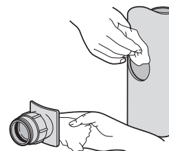
Fig.25b Cleaning mating surfaces
