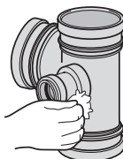
Fig.24d Removing excess cement
