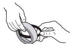
Fig.3b Fitting seal ring
