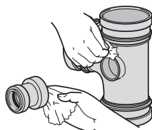
Fig.24a Cleaning mating surfaces
