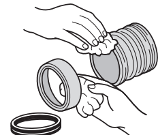
Fig.3a Cleaning mating surfaces
