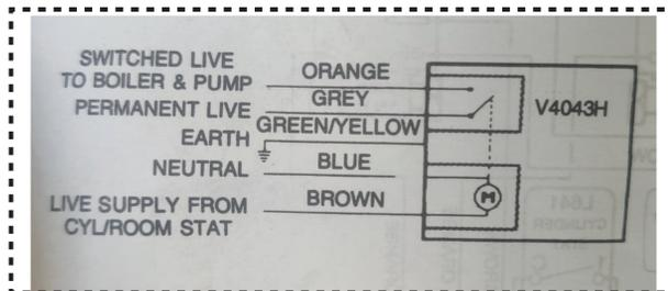
2 - This is the wiring diagram is it wired correct, because grey is the permanent live?
